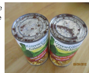
Rust caused by condensation
